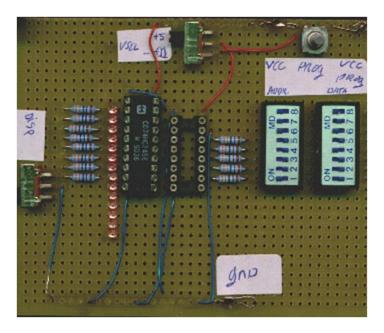
This page shows my home-brew BPROM programmer, constructed free-form on a bit of patchboard. The circuit itself is quite simple, using some leds to show the status of the BPROM outputs, and dip switches to enter the data and set the address lines.
